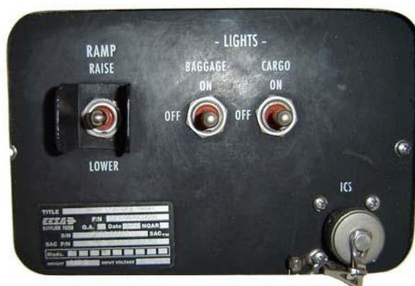
RAMP CONTROL PANEL
