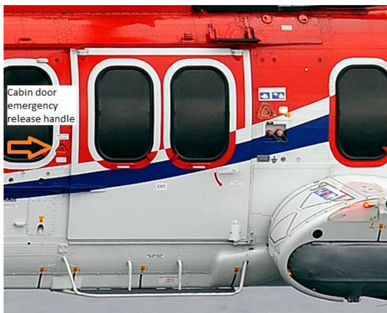
Opening the cabin emergency exit: Pull the handle in front of the cabin door until the door releases from the hinge tracks and falls free. (see fig)
