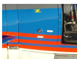
The battery is positioned on the left-hand side of the helicopter just forward of the pilot pedals behind this shield.
