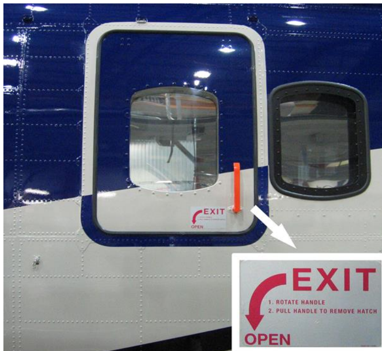
Fig. cabin emergency exit
