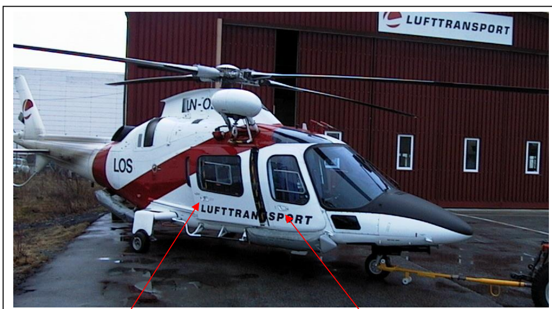
To open pilot door either side of helicopter: lift latch and open
