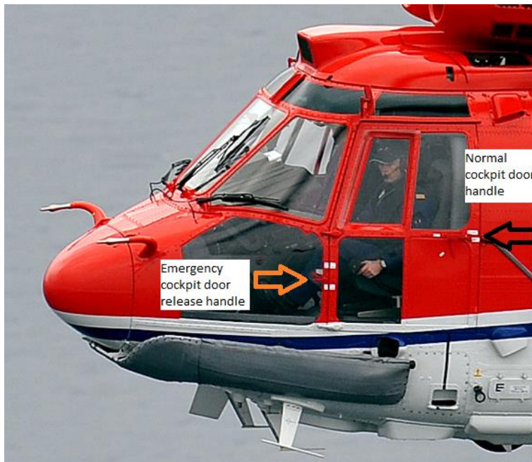
Opening the cockpit emergency exit: Turn the emergency release handle in front of the cockpit door downwards until the door releases from the hinges and falls free. (see fig.)
