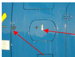
Grounding point for the pistol.
