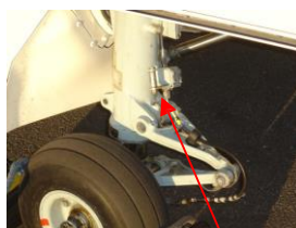
Ground the helicopter to this grounding point with the grounding wire.
