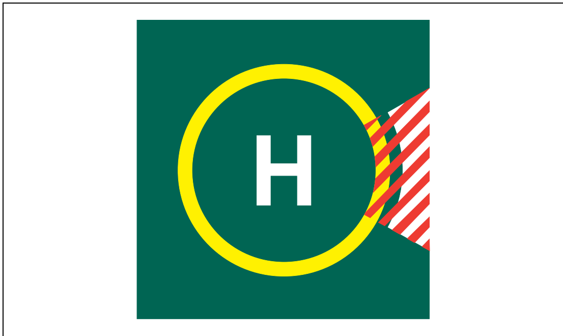
Figure 6 Example of Prohibited Landing Heading Marking
